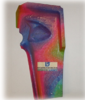
Figure 4. Stress Profile of hydroformed part.
