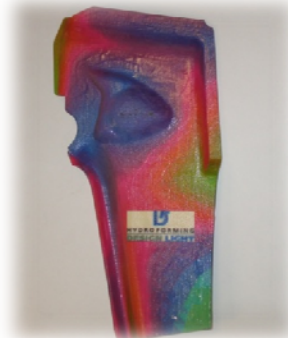
Figure 4. Stress Profile of hydroformed part.
