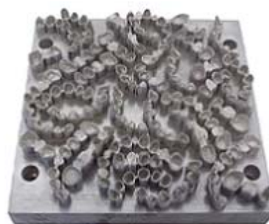
Fig. 4. Dental bridges produced by Hofmann Türk LaserCUSING® machine
