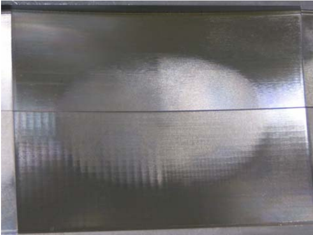
Figure 1: Some CAM systems cannot work to fine enough tolerances. In this example, Delcam's PowerMILL produced the smooth finish shown in the top half of the surface, while other systems produced the faceted surfaces seen in two sections of the lower half.
