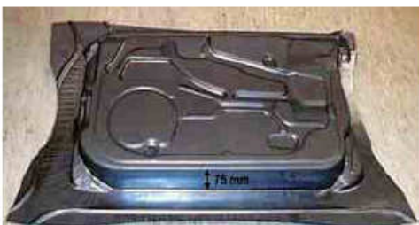
Figure 15 Schematic of the Dodge Neon door inner formed by the warm forming process [14].
