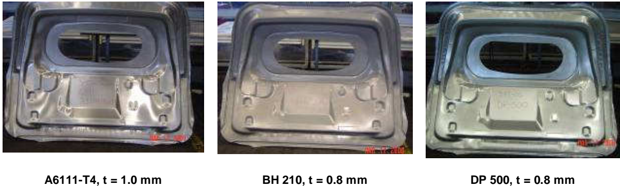
Figure 5 Schematic of the formed liftgate part from three different materials with different thicknesses in the same die by modifying BHF applied by the multipoint cushion system.
