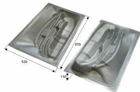
Figure 22 Schematic of the tooling and the inner door reinforcement formed from magnesium alloy at forming temperature of 400°C [22]
