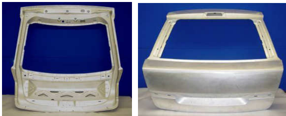
Figure 20 Schematic of the inner and outer panel of Malibu X deck lid formed by quick plastic forming processes [17]
