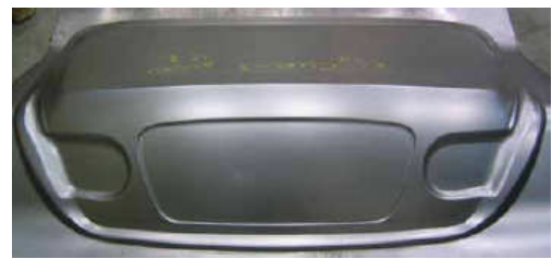
Figure 14 The formed part (trunklid – outer) using BHF variable in space and constant in time, predicted by FE simulation. The test was conducted at KIA Motors, S. Korea.
