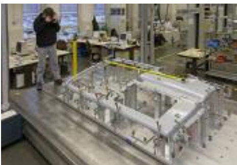
Figure 4. Creating a reference data set of a side panel with TRITOP
