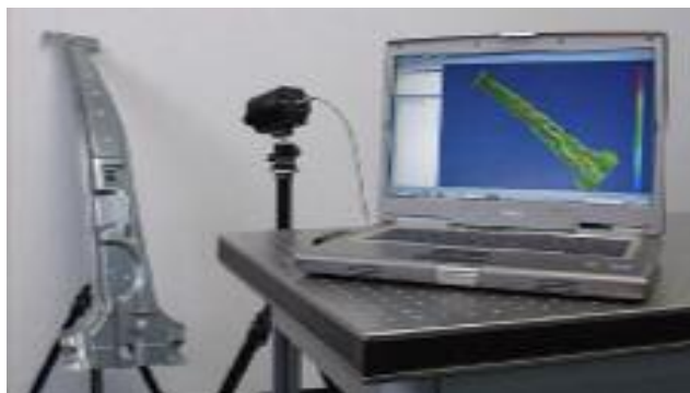
Figure 23: ARGUS system measuring; B-pillar with etched points showing major strain distribution
