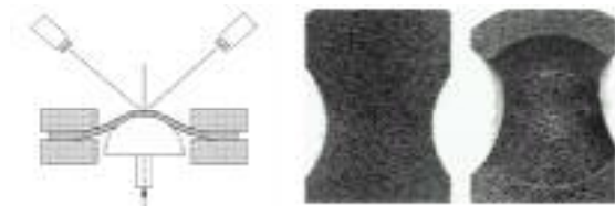
Figure 27: Principal setup & Figure 28: Nakazima specimen
